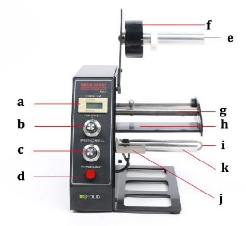
a. counter b. length control c. speed control d. power
